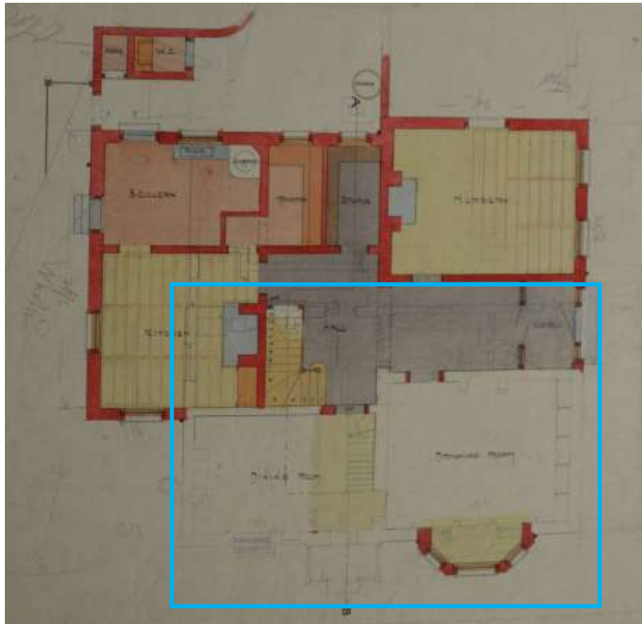
Figure 44: St Leonard's Priory – altered ground-floor plan, 1880 (north to left; new front entrance to right). The blue box identifies the principal rooms of the original plan.
